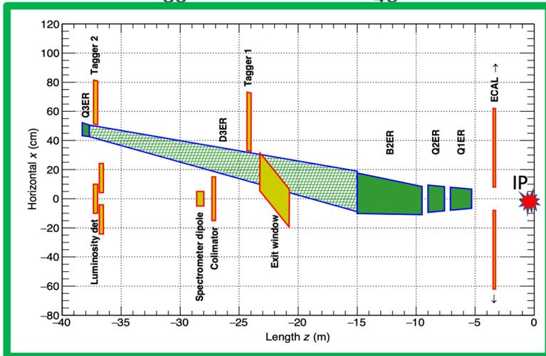
Extensive integration of forward and backward detector elements into the accelerator lattice
