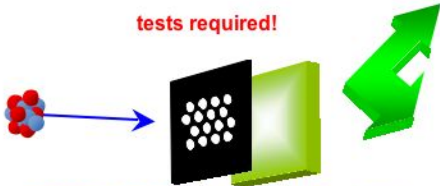
pepperpot mask, \varnothing 0.2mm holes
