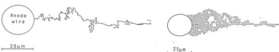
Fig. 5 Two dimensional display of a simulated drift process of one electron from starting point to anode wire surface.
