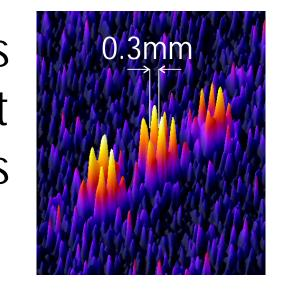
A secondary electron emission monitor was tested in collaboration with MSL in Stockholm. A collimator with 1 mm holes spaced 2 mm apart was used to test the resolution  $\bigcirc$ .
