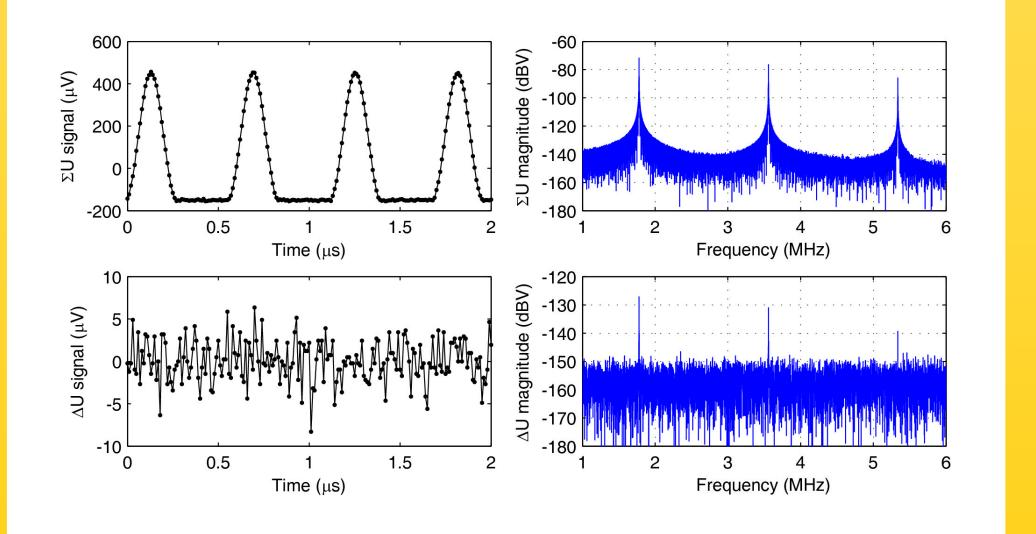
The main challenge for the pick-up system comes from the low number of particles generating very weak signals in the PU plates. In order to detect a beam displacement of 0.1 mm, one needs to be able to measure **300 nV** in a noisy environment of beamlines, vacuum pumps and electromagnetic fields.
