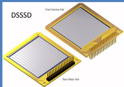
Double Sided Silicon Strip Detector
