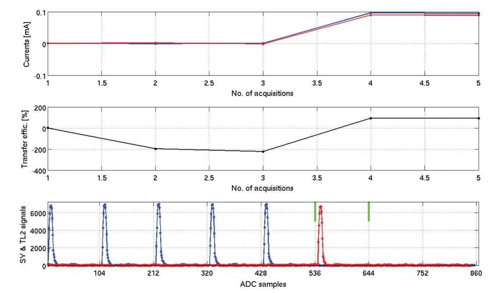
Finally, injection of single bunch. The injection efficiency is in this case properly calculated for three last acquisitions only.
