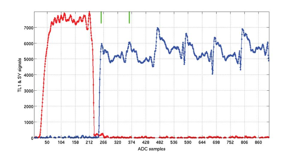
Injection of long pulse from TL1 (red) to booster (blue) at 1.1 mA. Booster revolution period can be easily observed. The excesive length of the pulse from TL1 can be seen.
