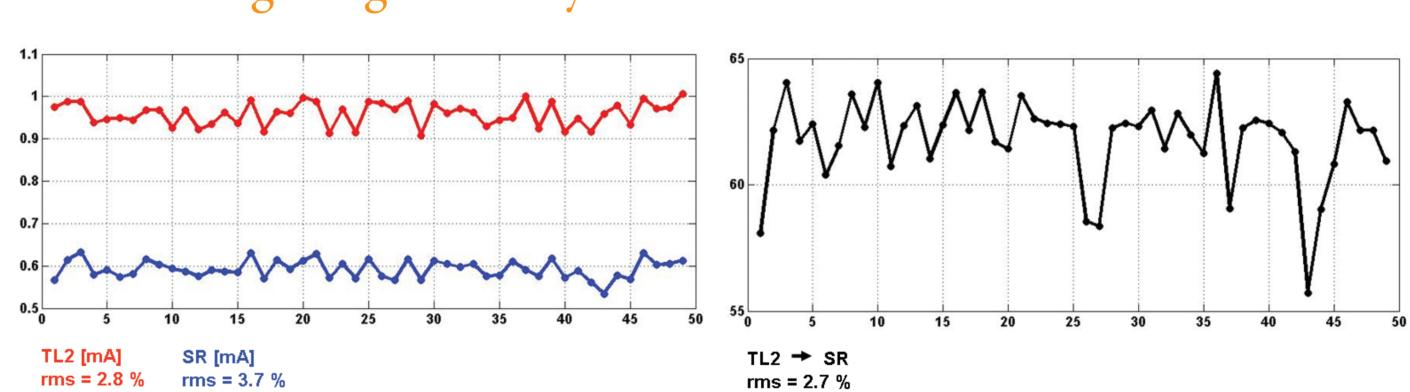
Red line shows the added current of each injection, as measured on stripline of TL2. At the same time (blue), the increase of the current after each injection was measured with regular Libera Brilliance devices, installed on pickup buttons on storage ring. The TL2 to storage ring efficiency (black, on right) is thus calculated in a very accurate way, with RMS of 2.7%
