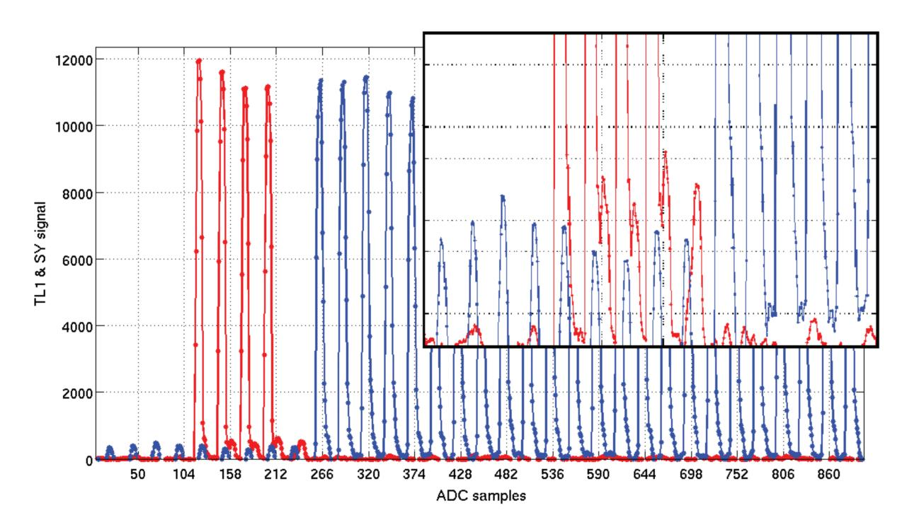
Injection of four bunches from TL1 (red) into the booster (blue), zoom at upper right. In the case above, bunches are not completely ejected from the booster, a small fraction of them surviving until the next injection. New bunches from TL1 overlap with small bunches from the previous cycle. This phenomenon was appearing randomly, and needs to be further investigated.
