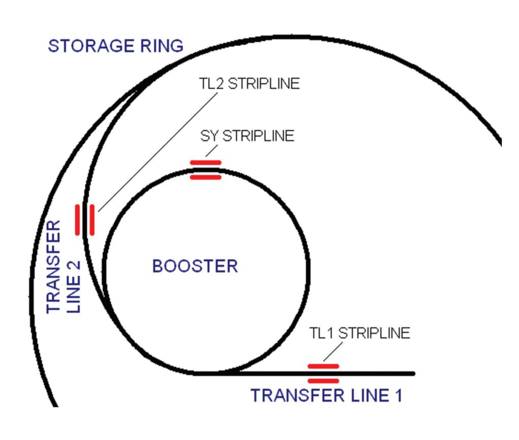
Test setup: measurements were performed in the ESRF injection system, where 3 Libera Brilliance Single Pass units are installed. The three units were connected to the striplines which are installed on the transfer line from the linac to the booster (TL1), booster (SY) and the transfer line from the booster to the storage ring (TL2).
