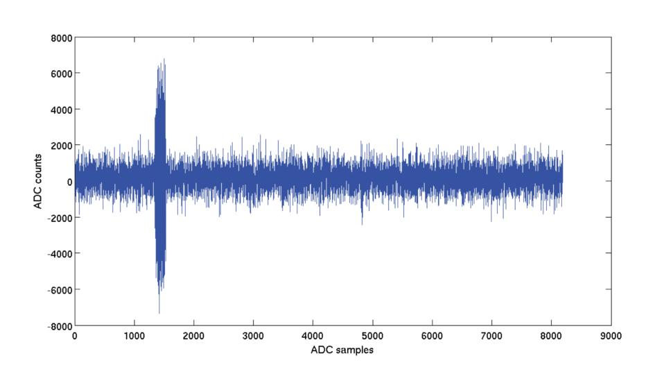
Signal to noise ratio at minimal booster current tested ( $\sim$ 30  $\mu$ A). The measurement is still reliable.
