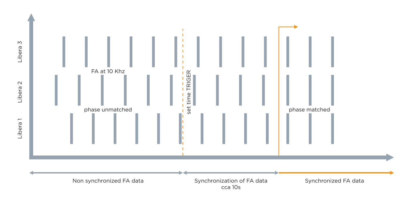
In addition to perfect synchronization of phase and frequency, the FA data packets are equipped with 16bit counters. These are reset on the set-time trigger to assure that the samples originating from the right moment in time are taken into account for the correction calculation.
