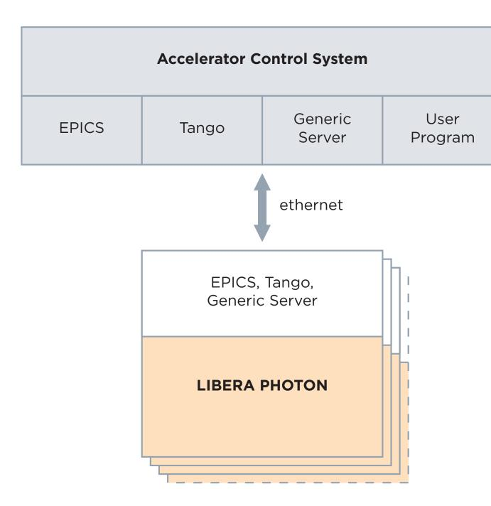
From the Control System point of view, the devices are very similar and it is thus easy to integrate Libera Photon in the Control system of existing Libera Brilliance user. Below is the schematic of the Libera Control System integration structure.
