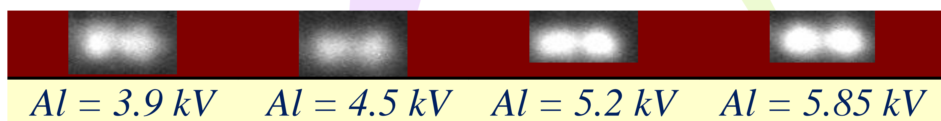
Figure 5: Recorded CCD images of the light produced in the F.S. for different Al plate voltages for 0.5 keV proton beam
