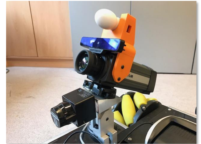
Vision system (2D Laser, radar, thermal and 2D-3D camera)
