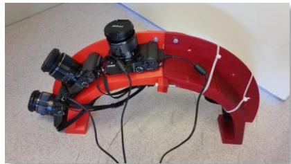
HD camera system for tunnel dome view
