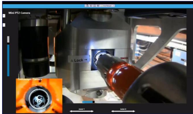
TIM Handling Radioactive Source for BLM Tests
