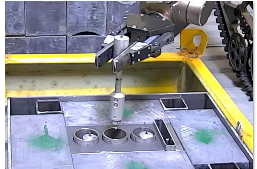
Radioactive sample handled by a robot
