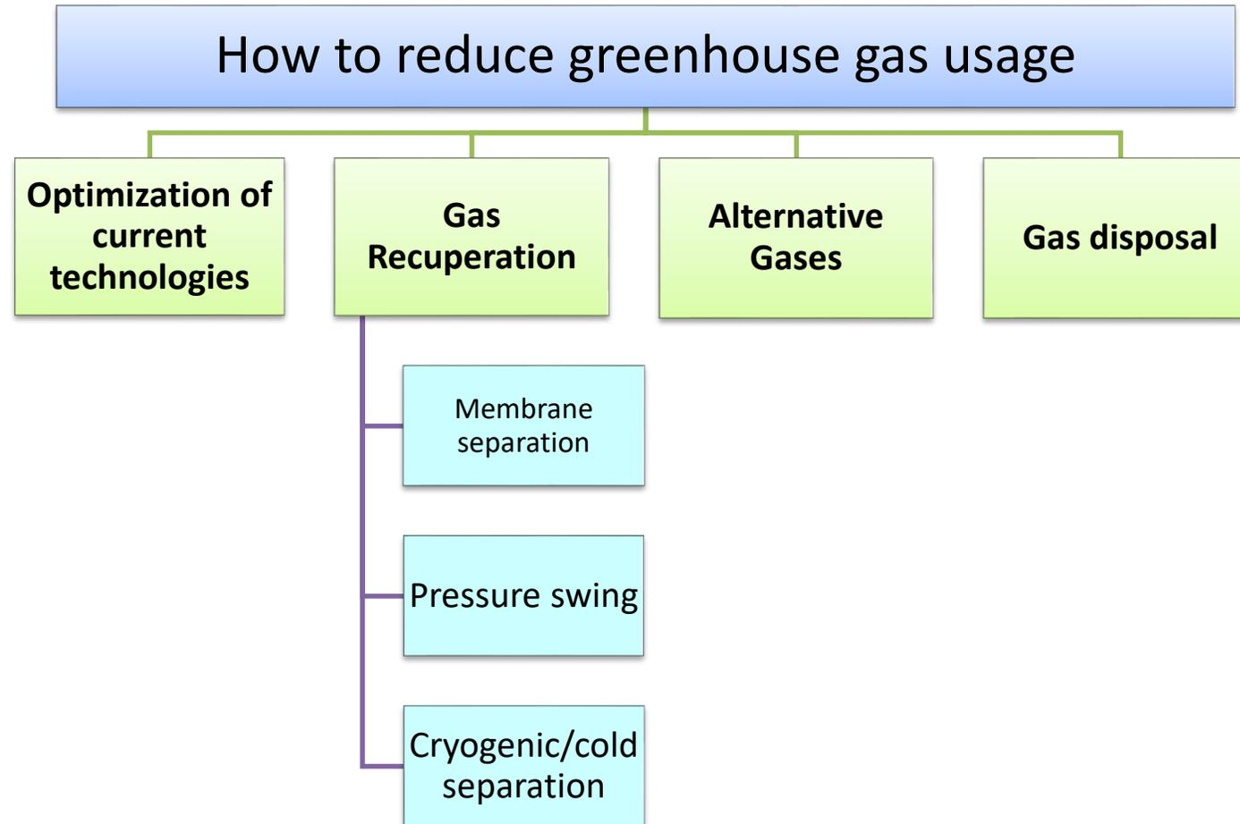
Possibility to recuperate a single gas component from exhausted mixture
