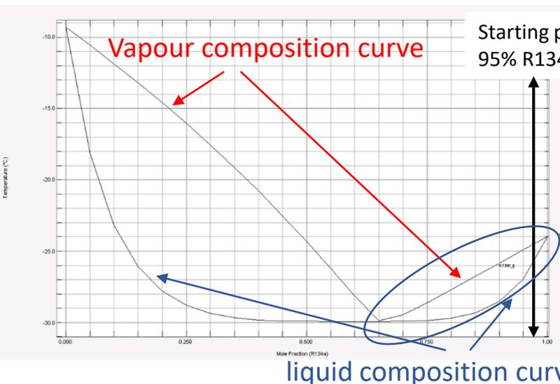
R134a/iC<sub>4</sub>H<sub>10</sub> remaining mixture is totally liquefied and it is sent to buffer at 5 °C:
