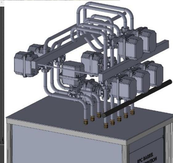
Detector pressure regulation was done using sensors at rack level:
