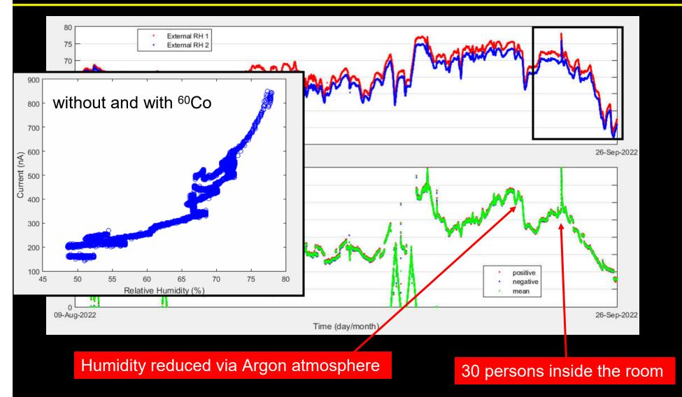
This can only come from leaks between the HV electrodes, through glass and epoxy surfaces!! We will work on it in the next prototypes, that are already in the oven..
