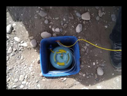
Gas bottle and distribution under ground to mitigate temperature effects. Probably we need to work on better solution due to condensation and tube material. We found some liquid inside the tubes, not clear what it is.!! Most probably water.
