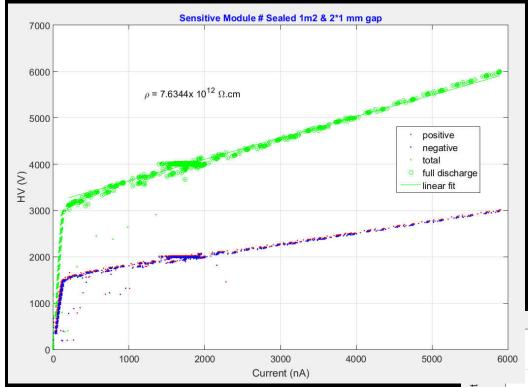
Argon permanent discharge. Very good gap uniformity. Able to extract correct glass bulk resistivity
