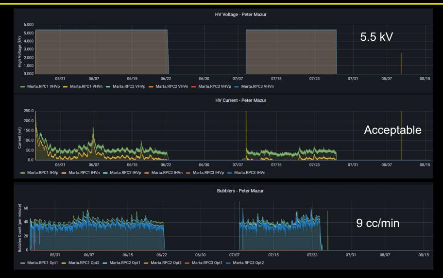
After 2.5 years seems to be all ok. Very high flow, not needed, misconfigured during installation!!
