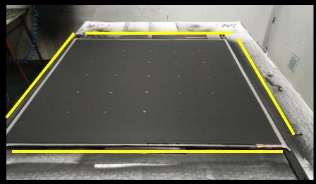
Leave 15 mm without paint to minimize leakage current and current flow over full glass paths, no paint in the spacer area
