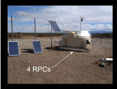
4 double gap RPCs with 1.2x1.5 m<sup>2</sup> active area underneath the tank. Deployed in November 2019, restarted in April 2022. After gas flowing for some days chambers were turn on.
