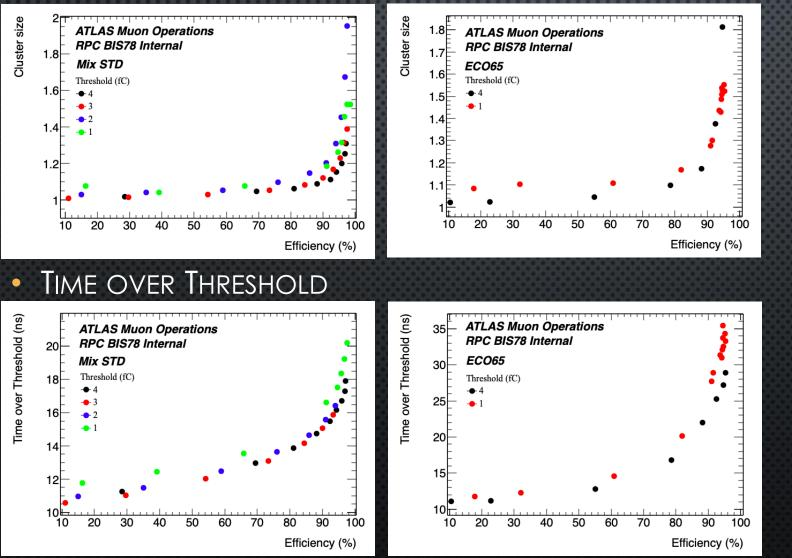
Culster size increases with both increasing applied HV and lowering the discriminator threshold.
