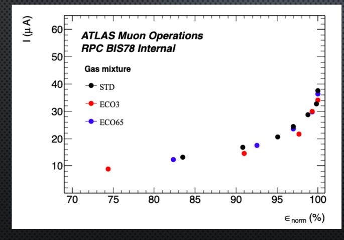
EFFICIENCY TO MIPS NORMALIZED TO THE PLATEAU ASINTHOTIC VALUE PHOTON INDUCED OPERATING CURRENT
