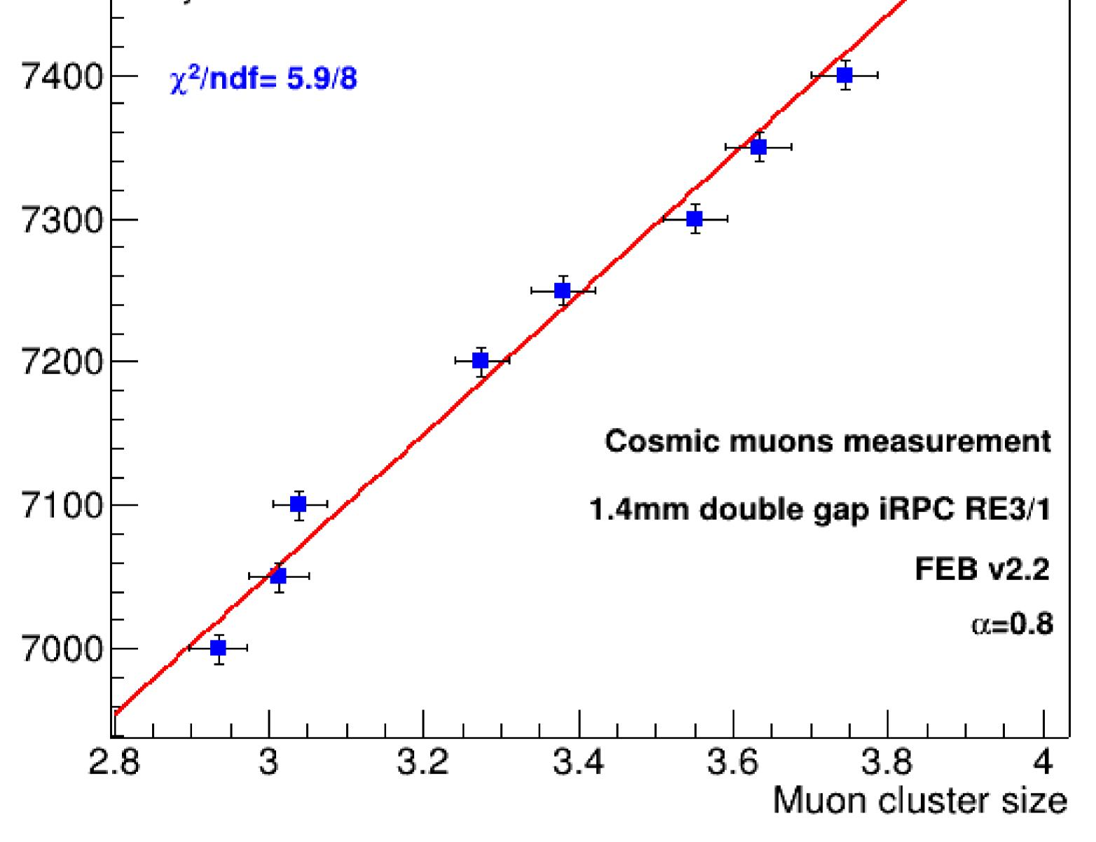
The figure shows the Selfconsistent extraction of the  $\alpha$ parameter from the cluster size measurement at different P values as described in step (6). We found that its value very close to the one of 2mm gap RPC chambers where the difference was 0.02 which gives a correction of 10 V for the effective WP of iRPC chamber.
