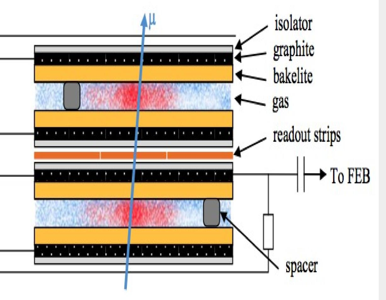
environmental pressure and temperature using the following equation (1) [4,5].  $HV_{app} = HV_{eff} \left[ (1-\alpha) + \alpha \frac{P}{P_0} \frac{T_0}{T} \right]$ (1)
