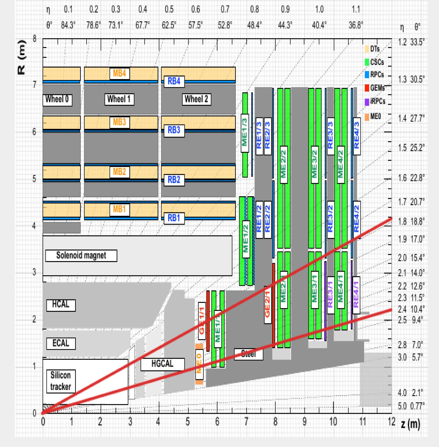
During the High Luminosity LHC phase (HL\_LHC), the instantaneous luminosity in the CMS experiment is expected to increase up to a maximum of  $5 - 7 \times 10^{34}$ cm<sup>-2</sup> s<sup>-1</sup> which is 5 times higher than LHC nominal luminosity. To deal with the expected high particle rate in the very forward region of CMS experiment, the new improved Resistive Plate Chamber (iRPC) will be installed in RE3 / 1 and RE4 / 1 regions [1].
