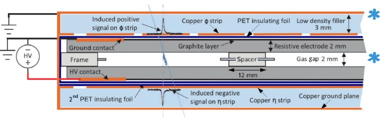
three concentric doublet layers, ~4000 m<sup>2</sup>,  $|\eta| < 1.05$ ~3700 RPC gas volumes of 2 mm width
