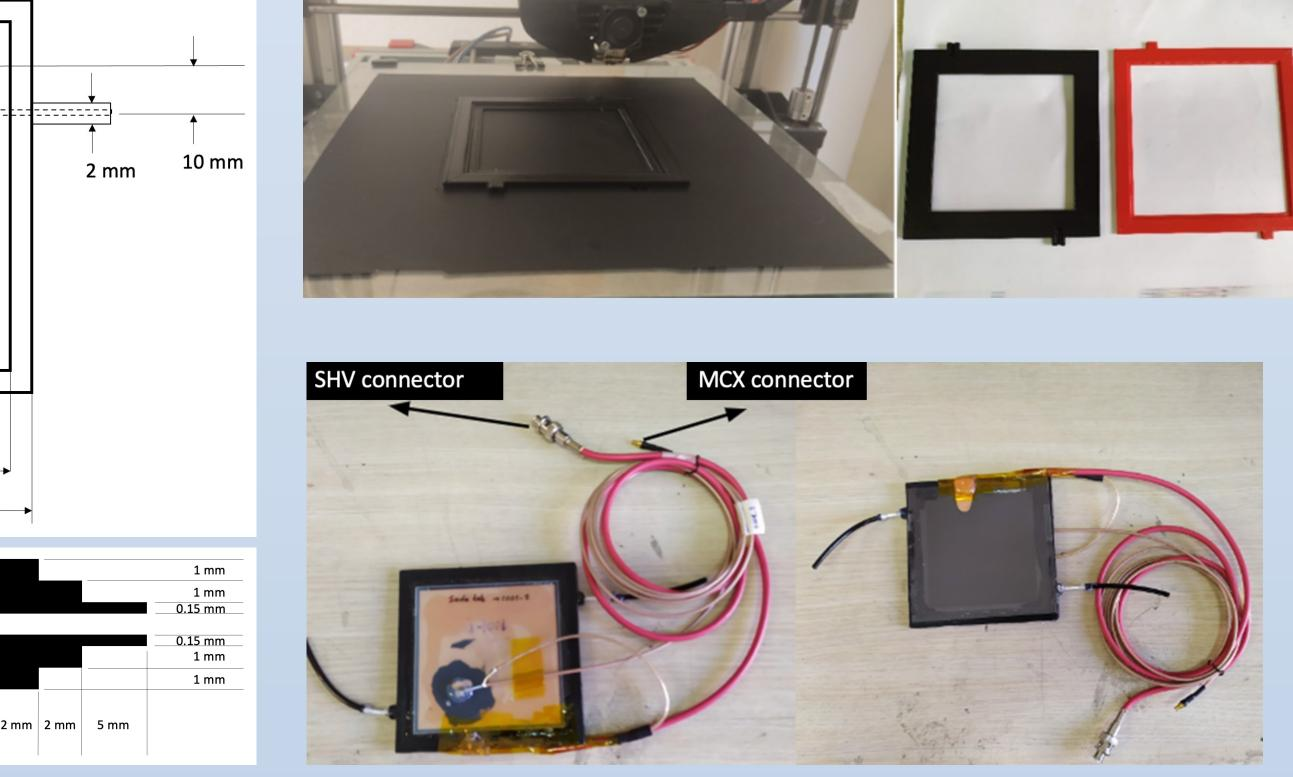
Sketches of the RPC frames are shown on the right (not to scale), as well as the pictures of 3D printing, pad boards and the assembled RPCs.
