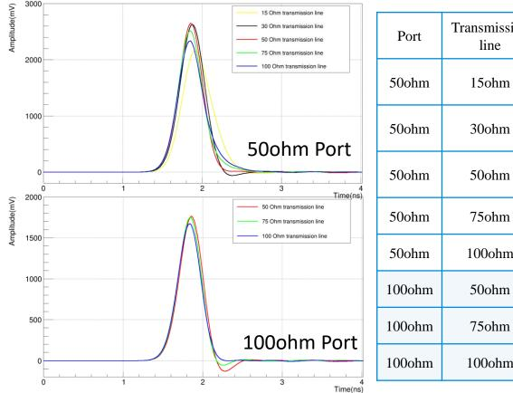
Transmission Rise Fall time time 276ps 372ps 267ps 247ps 246ps 264ps 307ps 261ps 370ps 100ohm 263ps 264ps 206ps 259ps 207ps 231ps 100ohm 259ps
