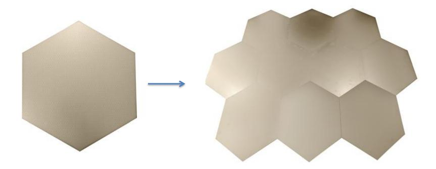
Large detection area can be instrumented by assembling easily many PCB.
