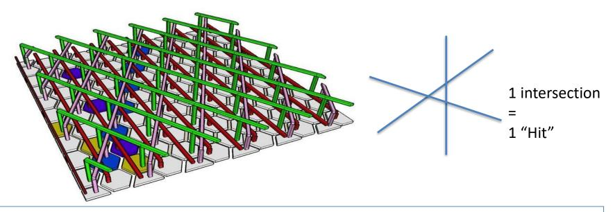
NXN  $\rightarrow$  3N : Reduction of electronic channels, power consumption and occupancy
