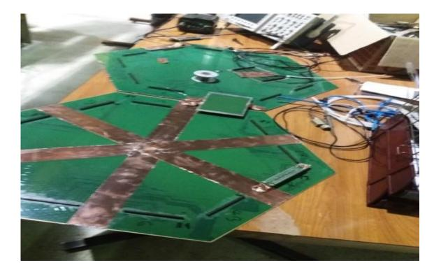
No signal loss was observed by injecting a signal on the furthest end of the first PCB and detecting it on the opposite side of the second one.
