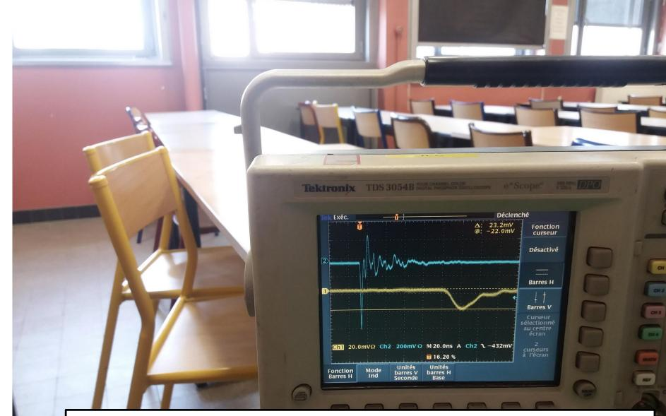
The shape of a RPC-like signal injected on one end and detected on the the opposite one ( > 7 m) is different but the charge loss is rather small).
