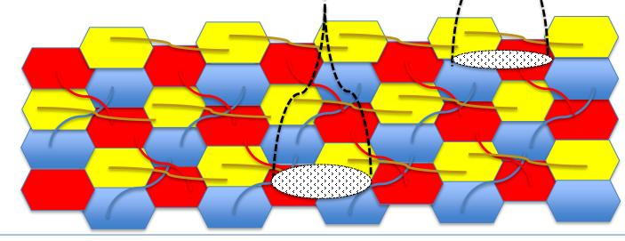
NXN  $\rightarrow$  3N : Reduction of electronic channels, power consumption and occupancy
