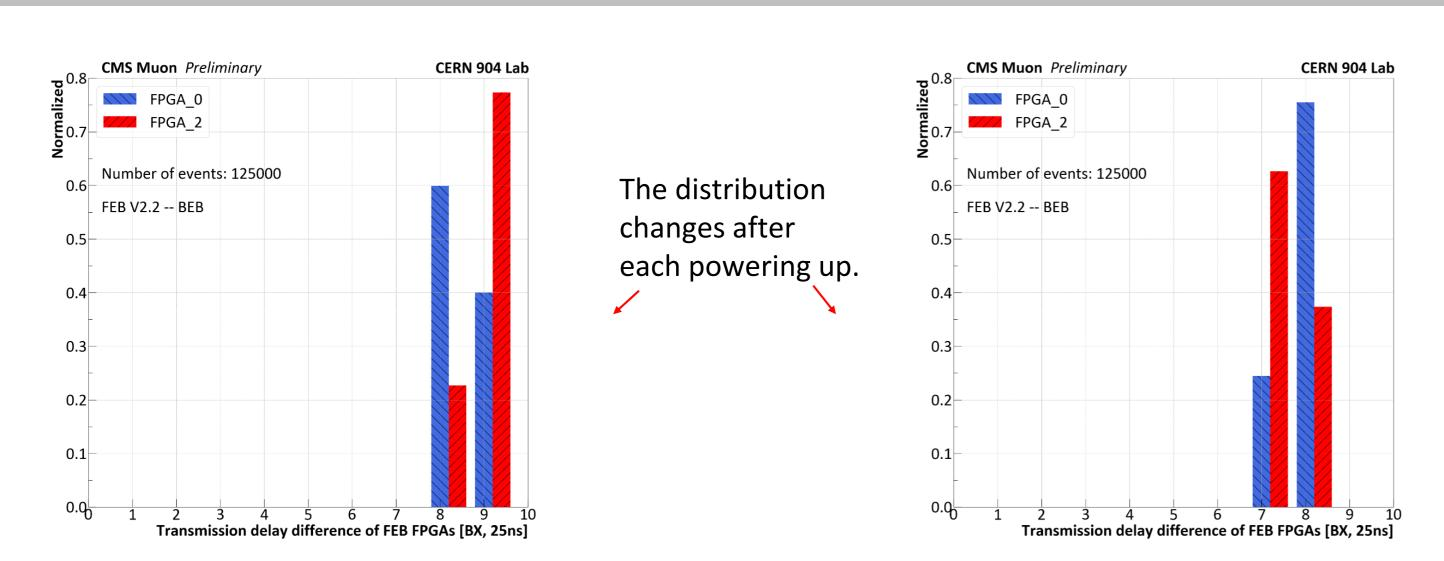
The transmission delay difference of FEB FPGA0/2 compared to FEB FPGA1 (0 BX point position). The data from FEB FPGA0/2 comes 7-9 BX later than FPGA1. It was caused by the serial links used for communication between three FPGAs and can be solved by implementing the IHEP proposal "Check-Sort-Push" mechanism.
