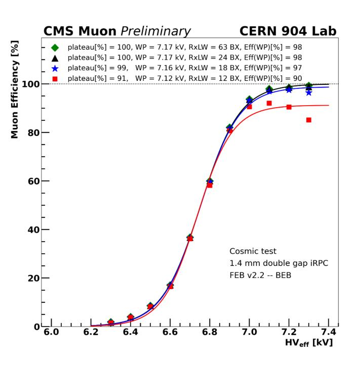
High voltage efficiency scan is a powerful way to verify the whole system efficiency When RxLW = 12 BX, the efficiency was not high. And it increases to 100% when the RxLW is 63 BX (test situation, at the cost of 1 link per BEB). This will be improved by implementing Check-Sort-Push mechanism (sorting in time sequence before sending) in FEB.
