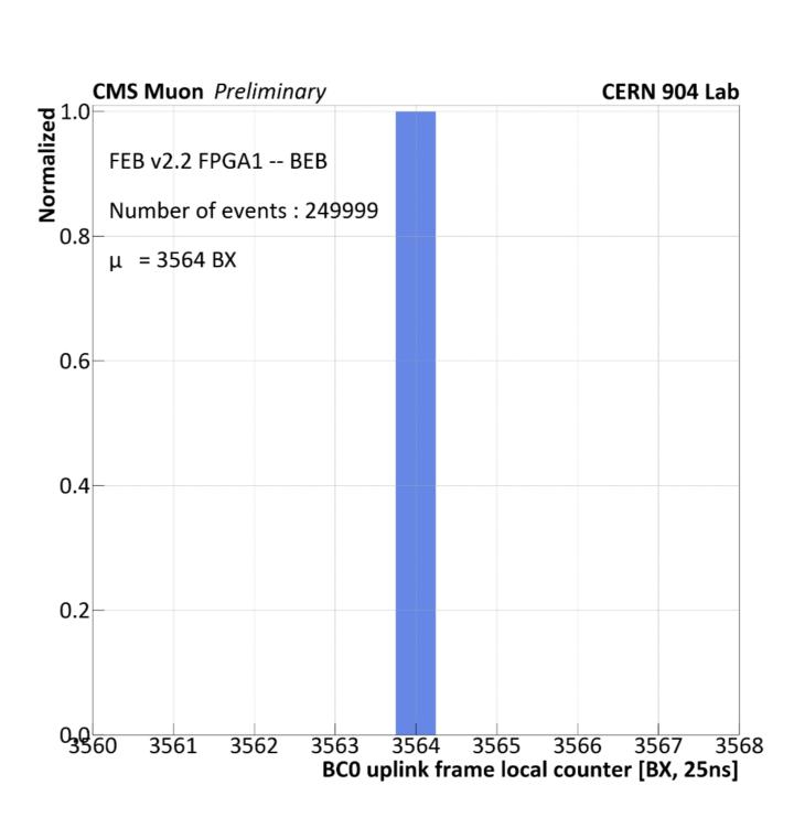
The FEB was connected to BEB via optical links and the fast control signal "BCO" need to be transmitted to FEB every 3564 BX. Then the FEB will perform TDC function on BCO channel and reply the BEB with its timestamp. The time interval between two BCO timestamp was measured 3564\*25ns (BX) as expected by the local counter in BEB.
