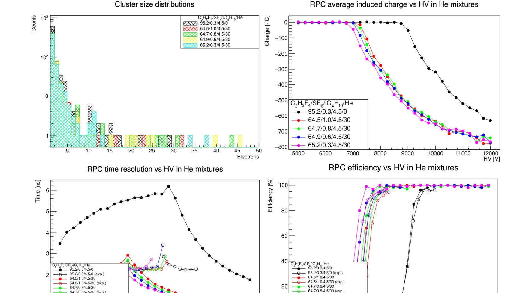
We compare the primary ionization clusters distribution for each gas mixture. We then integrate the current signal calculated in the readout for each event, the induced charge is registered, the efficiency is calculated as the number of events with a total induced charge greater than a 50 fC threshold. Finally, we calculate the time resolution as the FWHM of the arrival time distribution.
