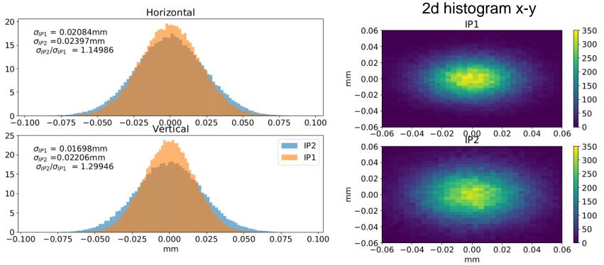
Tracking simulation: Ideal machine (beam 1) + trim of the
