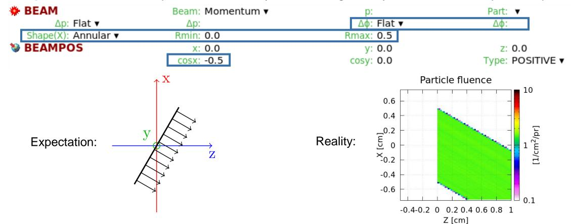
• Remember: the **BEAM** card sets the X-Y shape of the beam, which is not influenced by the beam direction set in the **BEAMPOS** card... so how can we rotate the beam?
