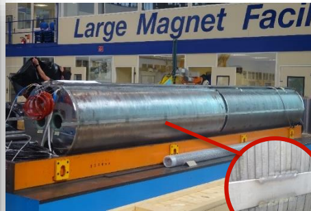
Backing strip welding
