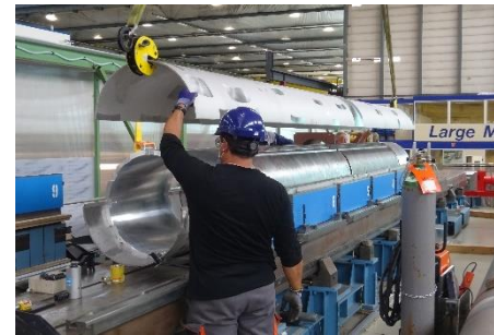
Upper shell installation
