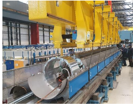
Transfer the magnet and the lower shell to the press conveyor
