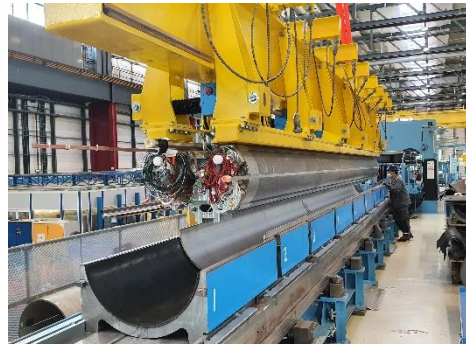
Transfer the magnet into the temporary shell
