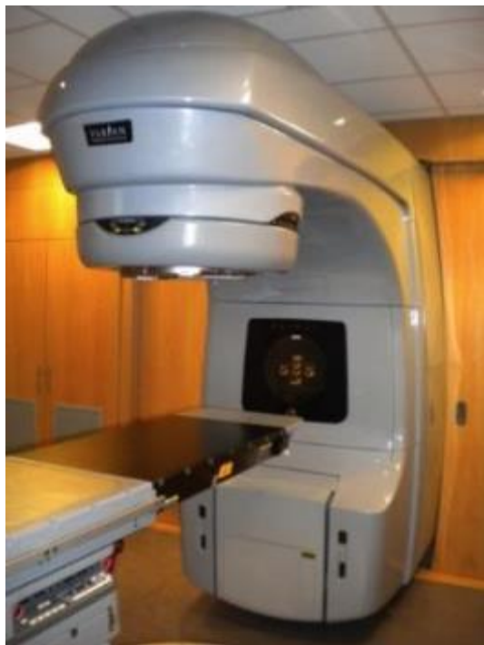
Electron Linac (linear accelerator) for radiotherapy (X-ray treatment of cancer)
