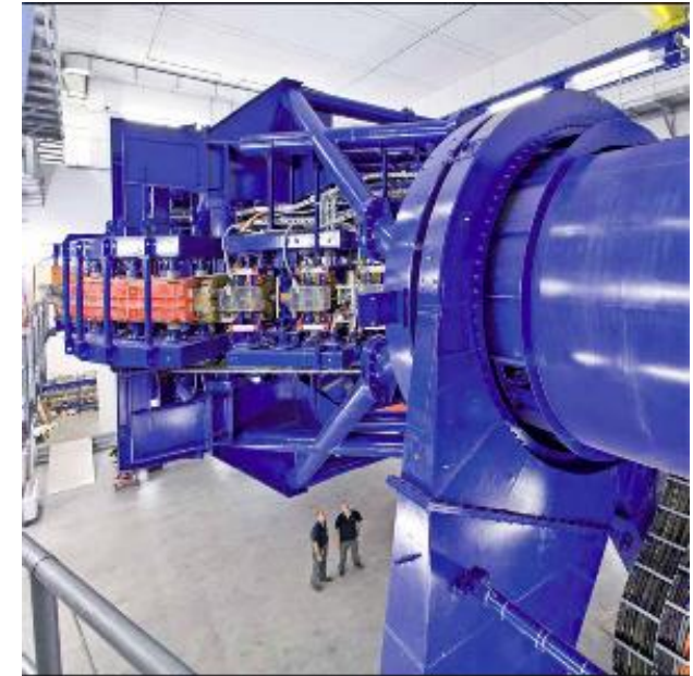
The ion gantry of the Heidelberg Ion Therapy facility: 600 tons
