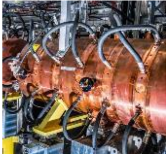
Multi-cell linac cavity (Linac4 120 MeV, 352 MHz)
