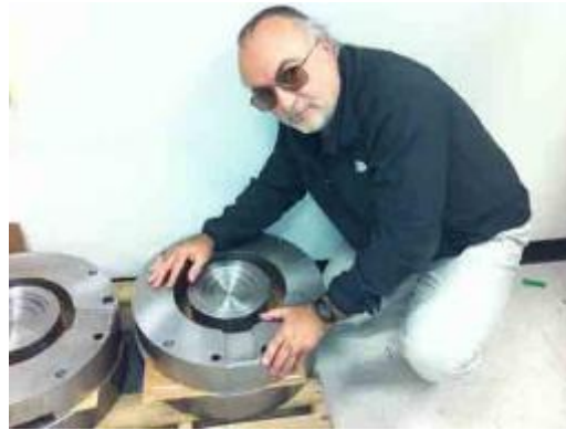
T. Antaya with steel pole and yoke pieces for the Ionetix, a 12.5 MeV cyclotron called the Isotron. (Courtesy of Ionetix)
