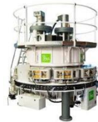
The IBA Rhodotron for production of intense electron beams
