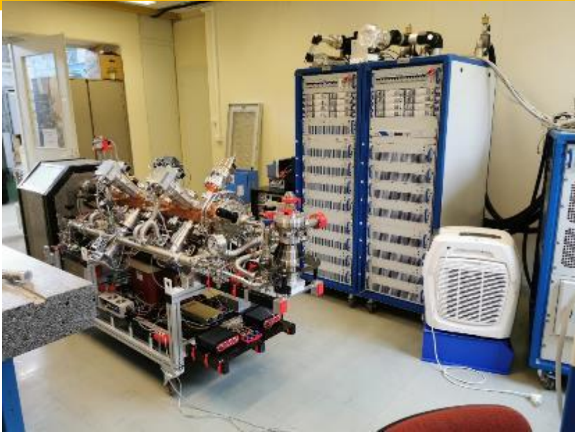
The CERN-INFN high-frequency RFQ-based system for artwork analysis: 2 MeV in 1.4 m 2 , less than 250 kg, 3 electronic racks
