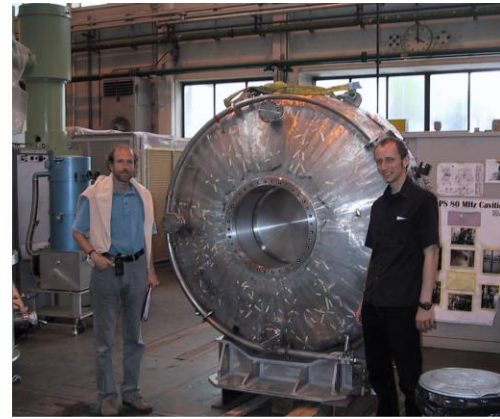
Single-gap cavity 88 MHz
