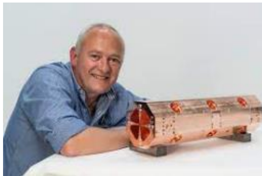
The CERN-INFN high-frequency RFQ-based system for artwork analysis: 2 MeV in 1.4 m 2 , less than 250 kg, 3 electronic racks
