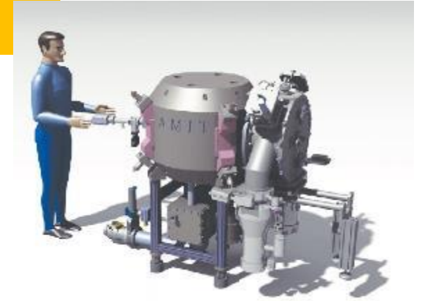
The AMIT superconducting cyclotron of CIEMAT (Spain), 8.5 MeV, 10 uA, in construction
