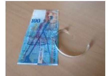
100 CHF (=100$) of YBCO HTS tape built by Bruker HTS for CERN
