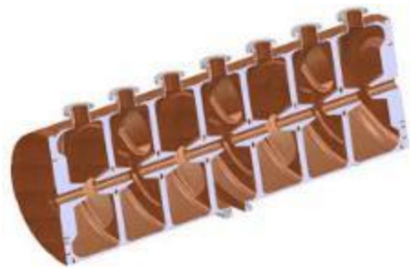
Multi-cell linac cavity (Linac4 120 MeV, 352 MHz)
