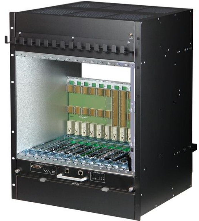
14-boards ATCA crate
