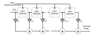
• Least Mean Squares (LMS) filtering algorithm is proposed to adjust the weigths of the FIR filter;
