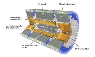
• In the Tile calorimeter (TileCal), the particle energy is absorbed (steel) and sampled by scintillating tiles.
