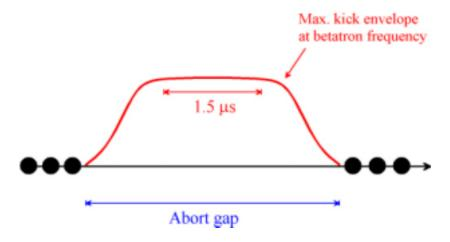
Figure: Envelope of the transverse damper kick inside the abort gap. The excitation frequency should be higher than the fundamental frequencies of 3 and 8 kHz (but smaller than 1 MHz) to spread out the tune in phase space and avoid that all beam hits the collimator in a too short time interval.
