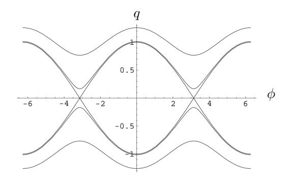
Phase space trajectories of particles with different q (maximum momentum deviation, normalised to the bucket height):
