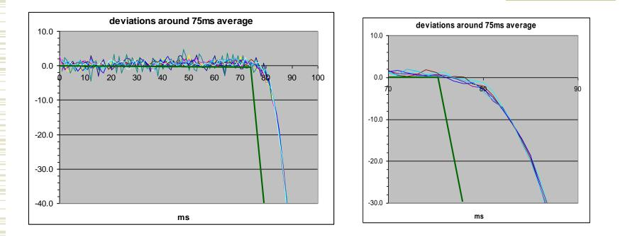
MSE Power Converter delay of output current with respect to the reference (due to filters).
