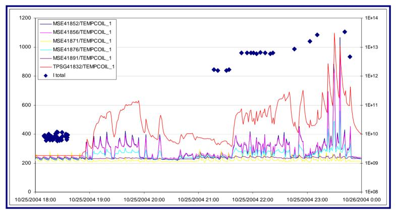
Conclusion : MSE temperature probes pick up beam signals with high intensity beam. Equipment expert disabled the temperature interlocks on the PLC side and extraction continued
