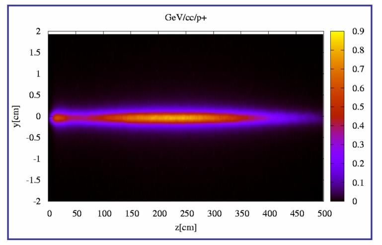
• A FLUKA model of the impact was made with the 1mm steel chamber and the calculated parameters (x' = 0.59mrad, sx = sy = 0.7mm, 3.4 1013 p+).
