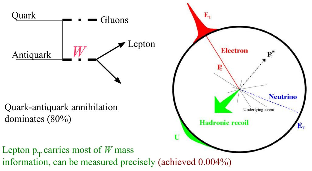
Initial state QCD radiation is O(10 GeV), measure as soft 'hadronic recoil' in calorimeter (calibrated to ~0.2%)
