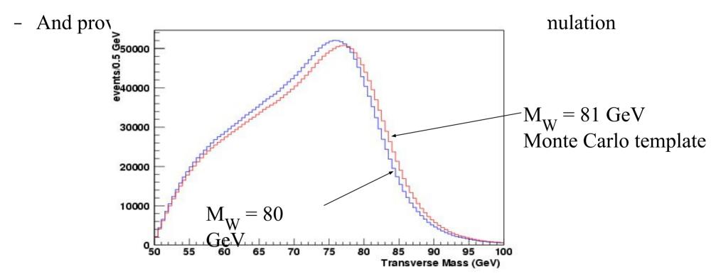
We will extract the W mass from six kinematic distributions: Transverse mass, charged lepton  $p_T$  and missing  $E_T$  using both electron and muon channels
