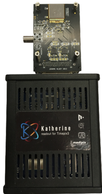
Figure: HR GaAs:Cr-Timepix3 detector with readout interface Katherine.
