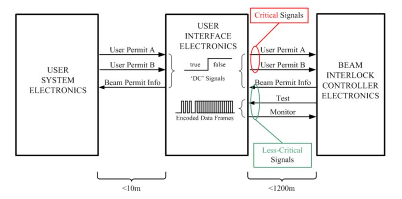
All links designed to be almost 100% testable from end to end of BIS Using Built-In Test Mode
