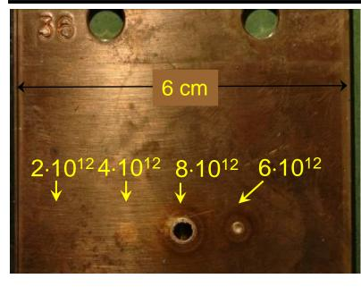
0.1 % of the full LHC beam  $8.10^{12}$  protons  $\sigma_{x/y} = 1.1$ mm/0.6mm
