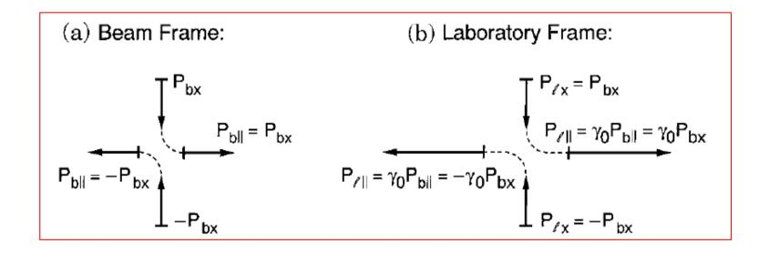
While the total momentum in the collision is preserved, the two particles emerge from this collision with opposite longitudinal momentum components that are larger by the factor  $\gamma_0$  than the original transverse momentum component before the collision.
