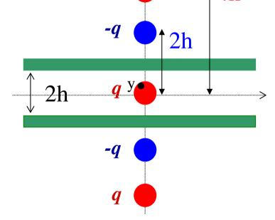
For d.c. or slowly varying currents, the boundary condition imposed by the conducting plates does not affect the magnetic field. We do not need "image currents "As a consequence there is no cancellation effect for the fields produced by the "image" charges.
