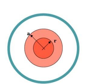
In the case of cylindrical charge distribution, and  $\gamma \rightarrow \infty$ , the electric field lines are perpendicular to the direction of motion. The transverse fields intensity can be computed like in the static case, applying the Gauss and Ampere laws.
