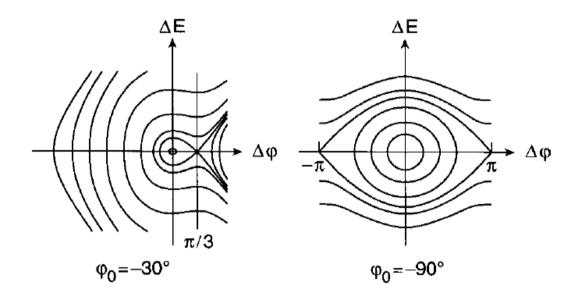
$$\Delta E_{\text{max}} = -\Delta E_{\text{min}} = 2 \left[ \beta_0^3 \gamma_0^3 \frac{\lambda}{2\pi} mc^2 q E_m (\varphi_0 \cos \varphi_0 - \sin \varphi_0) \right]^{1/2}$$
