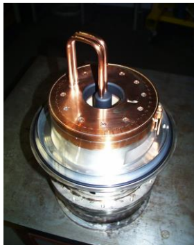
Main coupler PSI cyclotron
