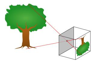
Figure 4.4: The principle of a pinhole camera.
