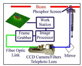
Figure 2.2: Experimental setup for three screen emittance measurement
