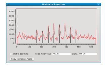
Figure 3.9: Projection of a pepperpot image cleaned of noise.
