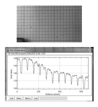
Figure 2.7: Calibration of readout setup using a mm-grid
