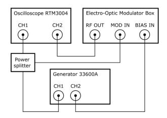
Figure 5.2: Connection diagram for the electro-Optic modulator test bench.
