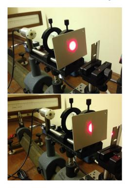
Figure 1.4: Beam imaged on white screen, without and with knife-edge in beam
