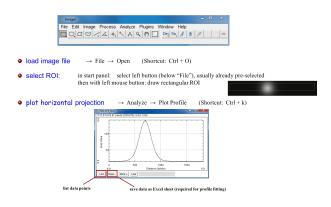
Figure 2.5: Selection of beam profile data for fitting.
