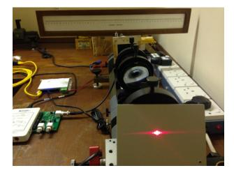
Figure 1.8: Single slit diffraction pattern.
