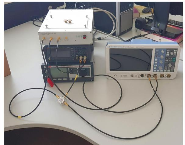
Figure 5.1: Electro-Optic modulator test bench.
