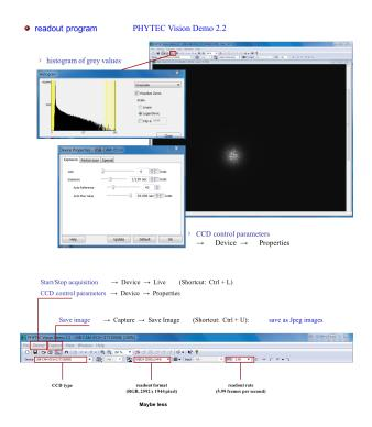
Figure 2.4: CCD control and readout.
