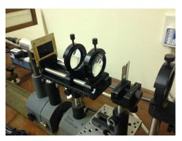
Figure 1.9: Filter inserted in front of photodiode.
