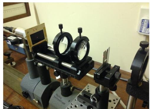
Figure 1.9: Filter inserted in front of photodiode.
