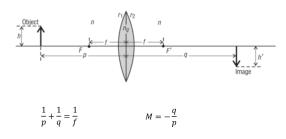
Figure 4.1: Imaging using a single lens.
