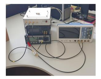
Figure 5.1: Electro-Optic modulator test bench.
