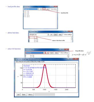
Figure 2.6: Gaussian fit to profile data.
