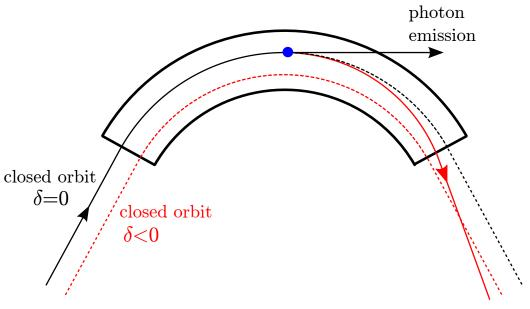
The beam eventually reaches an equilibrium distribution determined by a balance between the radiation damping and the quantum excitation.
