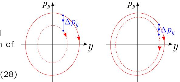
The amplitude of the betatron oscillations of a given particle can be characterised by the *betatron action*:
