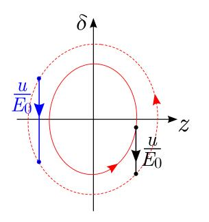
The change in the synchrotron amplitude of a particle when it emits a photon depends on the energy of the photon and on the synchrotron phase of the particle at the point of emission.
