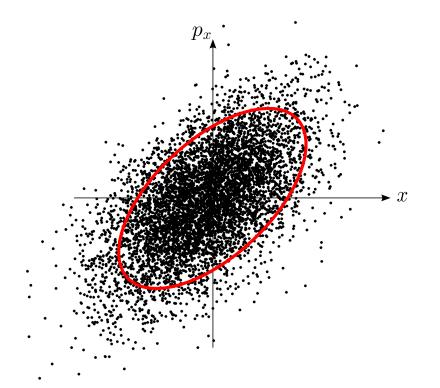
With some approximations, the emittance of a beam remains constant as the beam moves around a storage ring.
