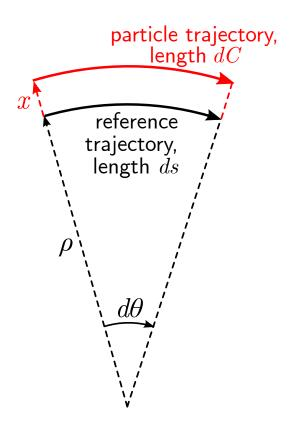
We have to take into account the fact that the field strength in a dipole can vary with position. To first order in x we can write:
