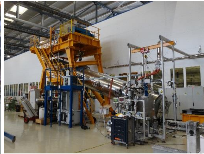
Second short (1.5 m) model magnet under preparation for test at CERN
