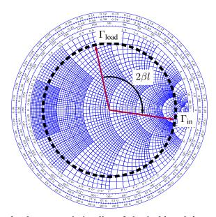
Fig. 53: Adding a lossless transmission-line of physical length l to an impedance  $Z_{\rm load}$
