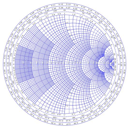
Fig. 45: Example of a typical *Smith* chart
