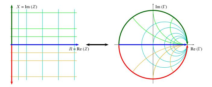
**Fig. 43**: Illustration of the *Moebius* transformation from the complex impedance plane to the  $\Gamma$  plane, commonly known as *Smith* chart.
