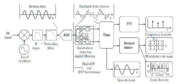
Fig. 18: Block diagram of a vector spectrum analyser
