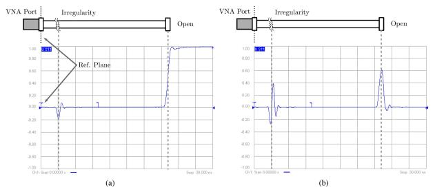
Fig. 32: Synthetic pulse measurement with a VNA: (a) step response; (b) impulse response.
