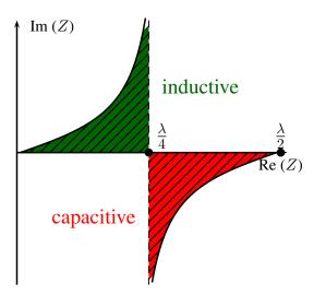
Fig. 54: Impedance of a transmission line as a function of its length l
