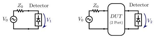
Fig. 27: A simple measurement set-up for the scalar transmission coefficient ( $|S_{21}|$ )
