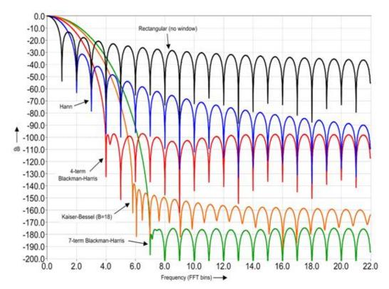
Fig. 35: Typical window functions to suppress strong sidelobes
