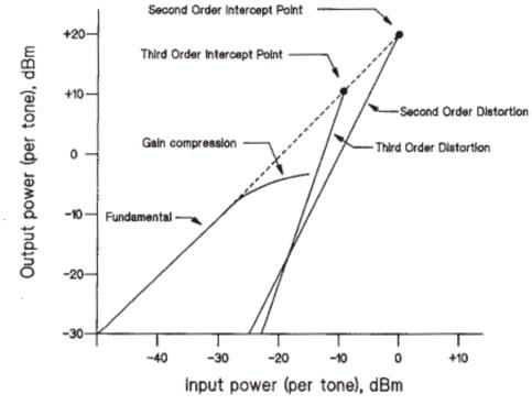
Fig. 11: Example for the 1 dB compression point [4]
