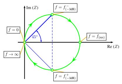
Fig. 61: Schematic drawing of the 3 dB bandwidth in the impedance plane
