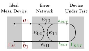
Fig. 38: Error model of a VNA. The parameters  $e_{xx}$  of the error network are determined by the calibration procedure and used to determine the true (corrected) result ( $\Gamma_{\rm DUT}$ ) based on the measured result ( $\Gamma_{\rm M}$ ).
