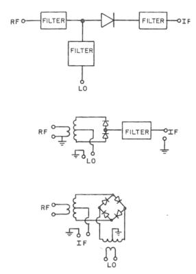
Fig. 6: Examples of different mixer configurations
