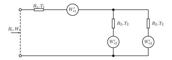
Fig. 22: Noisy one-port with resistors of different temperatures [6, 11]
