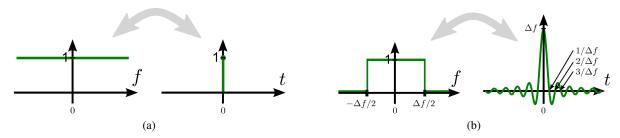
**Fig. 34**: (a) Infinite frequency span. (b) Limited frequency span. The limited frequency span  $\Delta f$  <sup>6</sup> of the VNA leads to "distortions" of the time-domain synthetic pulse measurement. The ideal response is convoluted with a sinc function, which characteristics depend on  $\Delta f$ .
