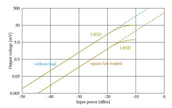
Fig. 5: Relation between input power and output voltage
