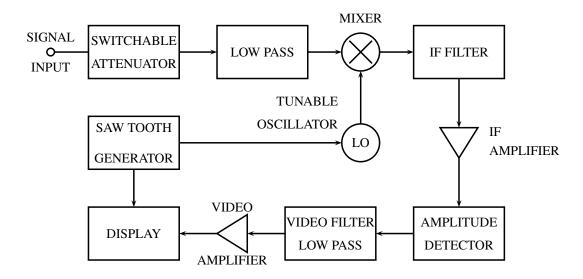
Fig. 16: Block diagram of a spectrum analyzer
