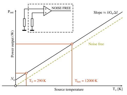
Fig. 24: Relation between source noise temperature  $T_s$  and output power  $P_{\text{out}}$  for an ideal (noise-free) and a real amplifier [7, 12].
