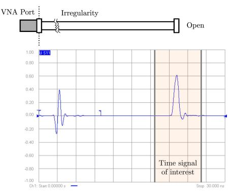
**Fig. 36**: Only the signal in a certain time window is of interest. After selection, the FFT of this window will be calculated. Here the real values of the synthetic impulse response are shown on a linear scale.
