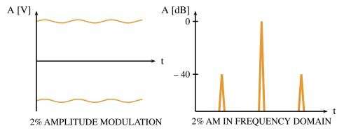
Fig. 14: Example of amplitude modulation in time and frequency domains
