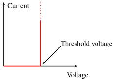
Fig. 4: The current-voltage relation of an ideal commutator with threshold voltage
