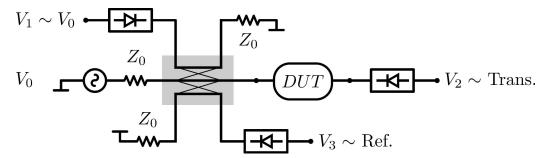
Fig. 30: Dual directional coupler in a network analyzer
