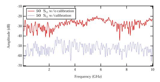
Fig. 39:  $S_{11}$  measurement of a 50  $\Omega$  termination with and without calibration. The calibration provides 20 dB improvement for this frequency range.
