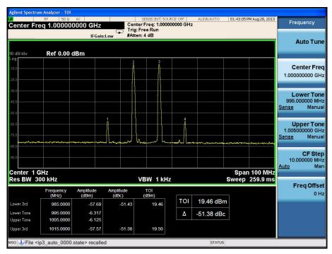
Fig. 12: An example of automatized TOI measurement
