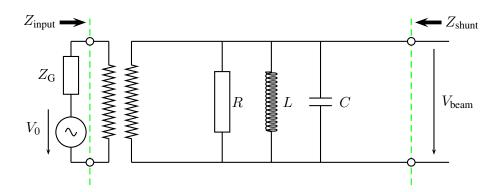
Fig. 60: Equivalent circuit of a cavity near resonance. The transformer describes the coupling of the cavity (typically  $Z_{\text{shunt}} \approx 1 \text{ M}\Omega$ , as seen by the beam) to the generator (often  $Z_G = 50 \Omega$ ).
