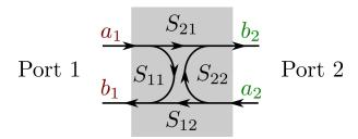
Fig. 26: All possible S-parameters of a two-port network
