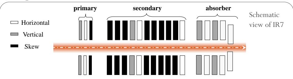
• Start aligning last horizontal collimator by setting it at  $5.7\sigma$  (nominal injection) => reference "beam edge"
