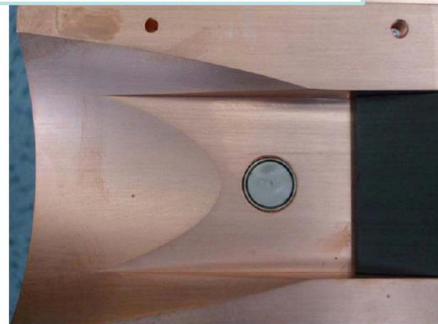
Button 1 at upstream port on D side Distance from Jaw face: 10 mm
