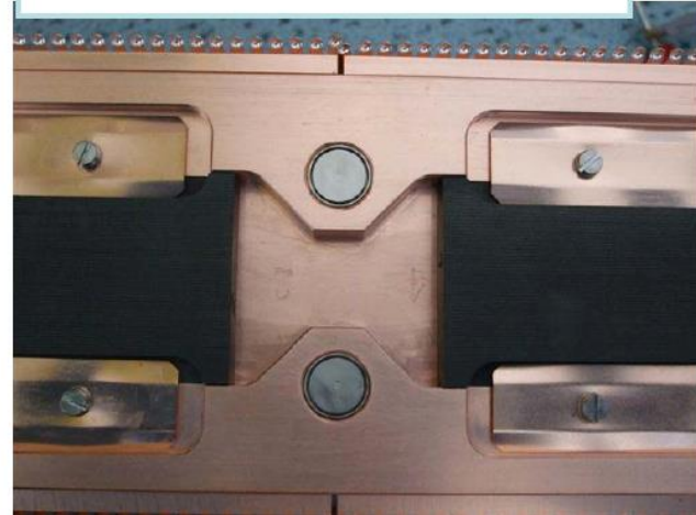
Button 10 at center of jaw on DB side Distance from Jaw face: 0.05 mm
