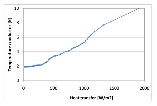
Steady-state heat transfer from conductor to bath through kapton (to be checked if for single cable or coil)
