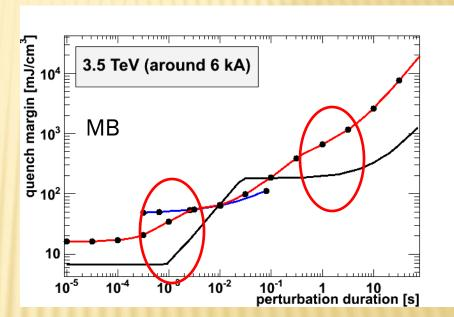
The 1-5s timescale is not limiting us now – we need to investigate 1 ms timescale – wire scanner test
