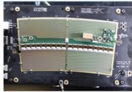
Irradiation of ITk Strip endcap modules (2 sensors) at DESY
