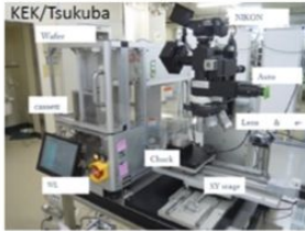
ITk Strip sensor probing at KEK
