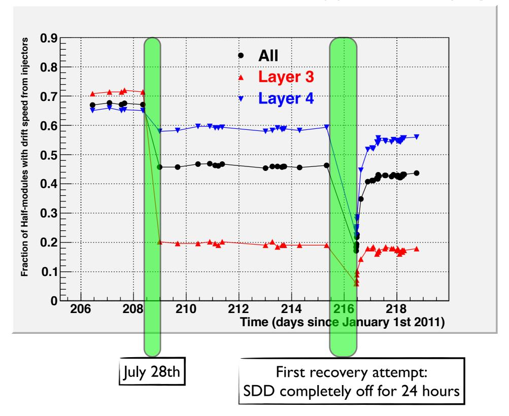
After the switch off the fraction of modules with drift speed from injector is unchanged
