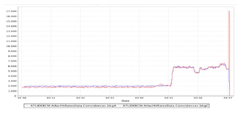
BCM background rates during the fill that show the adjusting of the beams and ultimately the spike in background activity.
