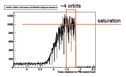
Low gain channels – far from saturation but substantial signal which looks to be exponentially increasing before beams were extracted (~140/1k).
