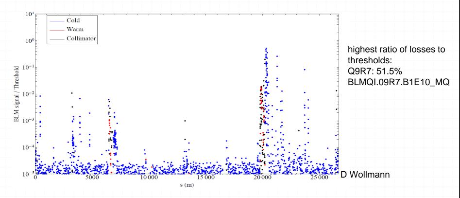
Fill #1: scale to assumed quench limit (x3 dump threshold) and assume constant loss rates factor of 3/0.515 ~=6 → inject 12 bunches (~ 1.6e11 charges)
