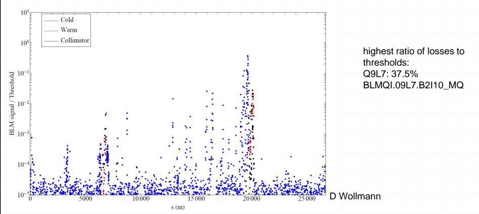
Fill #1: scale to assumed quench limit (x3 dump threshold) and assume constant loss rates factor of 3/0.375 = 8 → inject 16 bunches (~ 1.9e11 charges)
