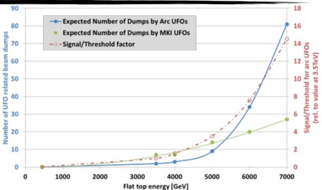
$\checkmark$  Mitigation = Increase BLM thresholds. Probe quench level in the ms scale
