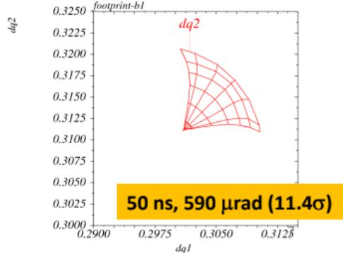
→ 100'000 turns DA simulation results vs Xangle confirming the “pathological tune footprint” (25 ns beam parameters,  $\beta^*=15$  cm, only sextupoles, LR and HO, no crab-crossing no field imperfection)
